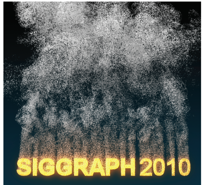
Figure 1: Simulation of rising bubbles generated around hot objects. The simulation was carried out using a 192 \times 256 \times 128 regular grid with a maximum of about 1,160,000 bubbles. The simulation took about 15 seconds per animation frame.
